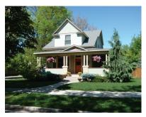
The use of compatible new awnings is encouraged as they are both traditional building elements and greatly enhance the energy efficiency of a home. An operable awning, as seen here, regulates internal temperatures throughout the year by providing shade in the summer while allowing solar access in the winter.
