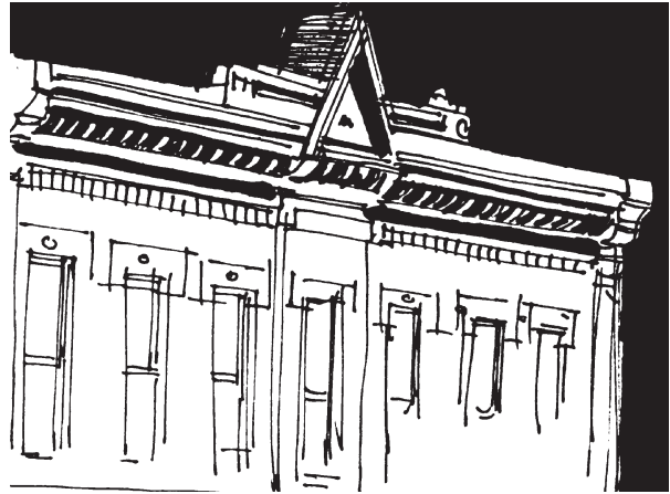
The Old Town design guidelines encourage reconstruction of missing elements, such as ornamental cornices.
