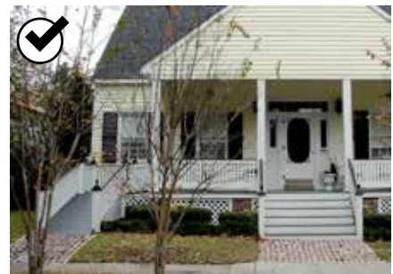
Avoid altering character-defining features when adding a ramp. For example, this ramp is set to the side, which maintains the character of the front steps.
