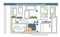
This diagram shows how a new infill project could work within the existing site without demolishing the original building. The new structure could step down in scale to transition smoothly to the original building. Parking consolidation between uses would allow for site enhancements.
