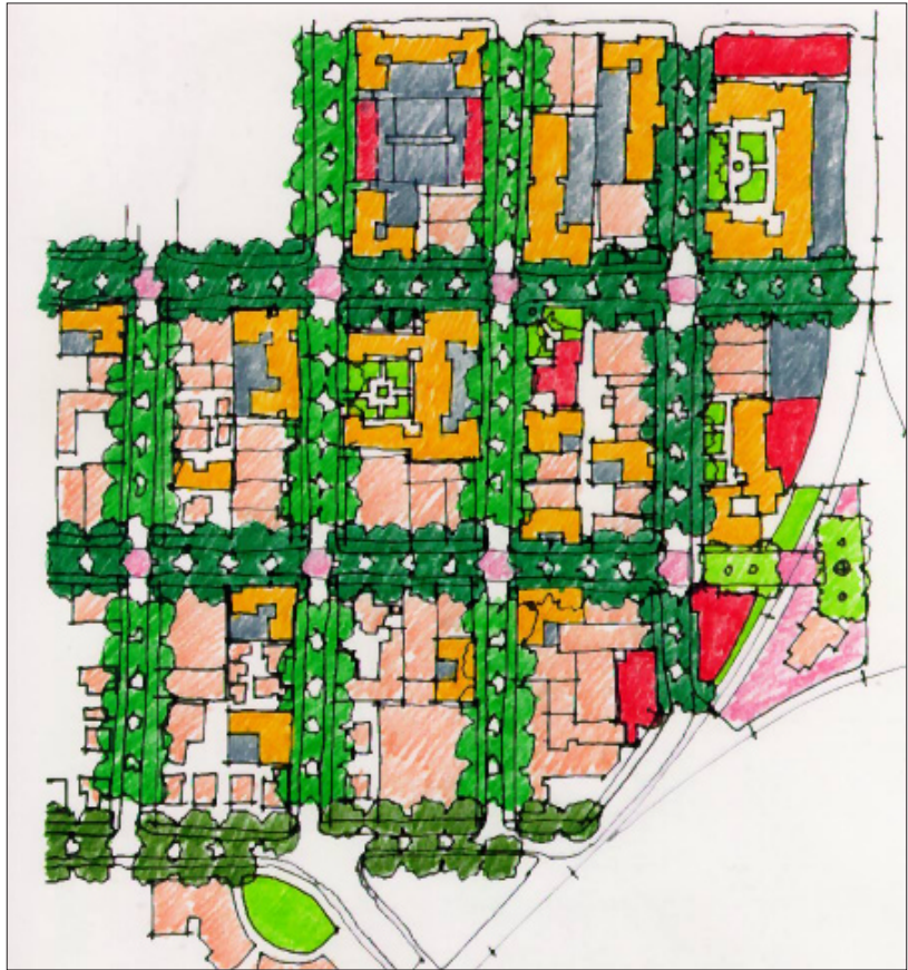
In an illustrative sketch plan for downtown Davis, California, three levels of streetscape design are differentiated with different shades of green. New infill is in yellow. Red buildings are part of the parking structure system.
